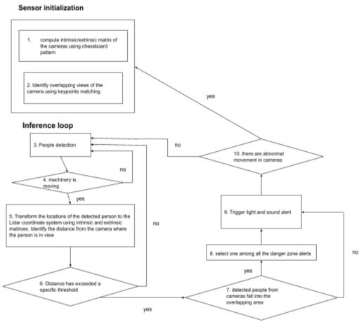
Fig 2: System Architecture of DZASS
